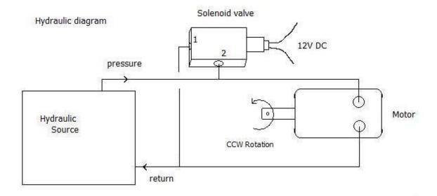
Note: Solenoid valve is normally open alowing bypass, supply 12V DC and valve closes forcing oil through motor.
